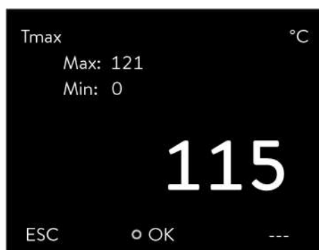
Fig. 30: Entering the new T_{max} value
