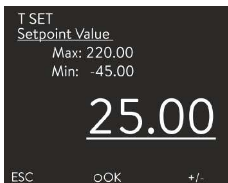
Fig. 32: Setting the set temperature
