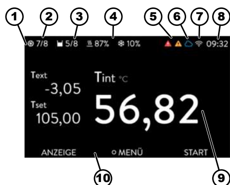
Fig. 24: Home window with status bar, temperature displays and softkey bar
